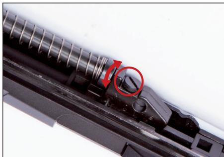
Gradually turn the lever from left to right and fire a round or two to see the effect. Continue to adjust until the BBs fly straight/horizontally. Perfect Hop-up is applied when the BBs fly straight.
